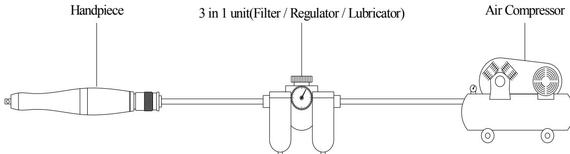
**Rules for Long Lasting and Performance Utilization:****Air Tools and the 3-in-1 units, Filter/Regulator and Lubricator**
