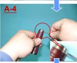
• Insert tool no. J-002 into the front cover, turn and remove the front cover.
