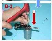
• Use tool no. J-8 to remove the bolt (#11)
