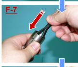
• Insert the turbine set into the rear body.
