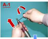
Use the Hex Key to remove the front screw and take out the tools holders
