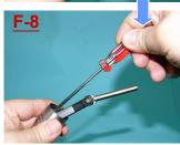
• Use tool no. J-32 to tighten the screw.
