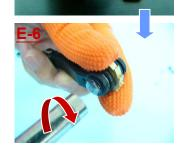
• Use tools no. J-34 to tighten the nut, same for both side.
