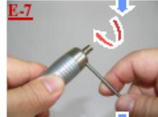
• Insert 3 mm round point on the nut cover ◦ And screw it ◦
