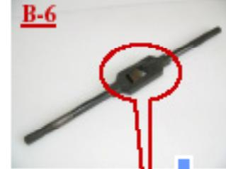
• Use the hand too to disassembly the front of main shaft
