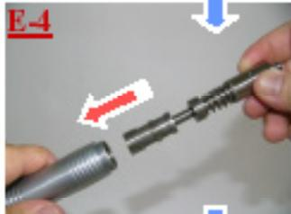
•Install the filling piece, as well as the slippery set, inner tube, and inspect whether skids smoothly ◦
