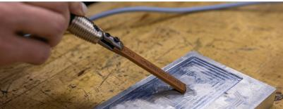
Manufactured using premium aluminum oxide grain, the AS-9 PLUS produces wider scratches on the mold surface which results in an overall smoother and more brilliant finish. Currently available in grits 320-800 and in a variety of our most popular sizes.
